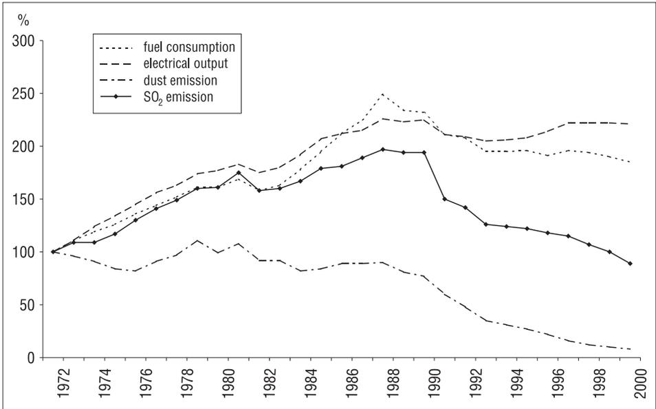
Fig. 1. Pollutant Emissions in Public Power Utilities vs. Fuel Consumption and Electricity Generation (1971=100)
