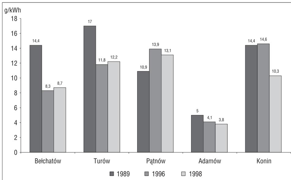
Fig. 4 Unit SO<sub>2</sub> Emissions in Brown-Coal Fired Plants in 1989, 1996 and 1998.
